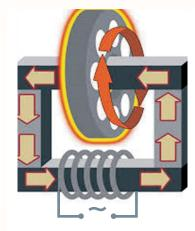
The proper mounting is the induction heating for heating the bearings having straight bore to mount the bearings onto the shaft.
